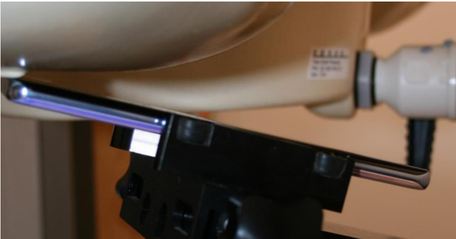
The tilt cheek position for phone only. The position is same for testing with the E-smog.
