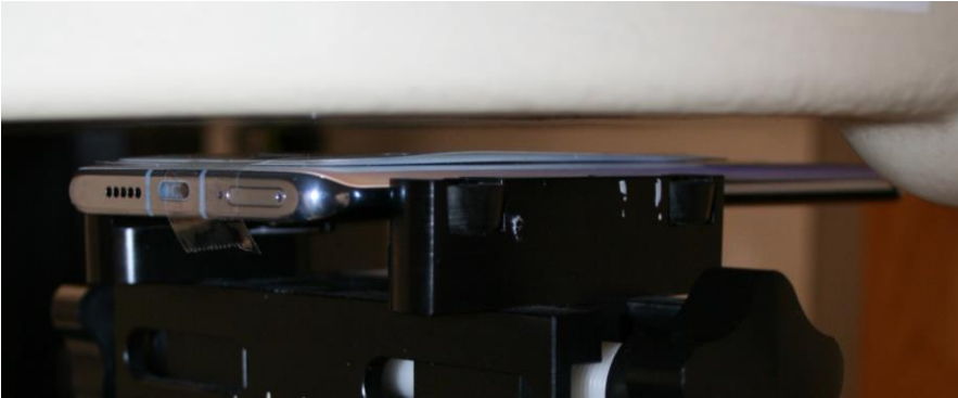
Back side of the device with E-smog against the flat phantom with 5mm separation
