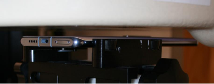
Back side of the device against the flat phantom with 5mm separation
